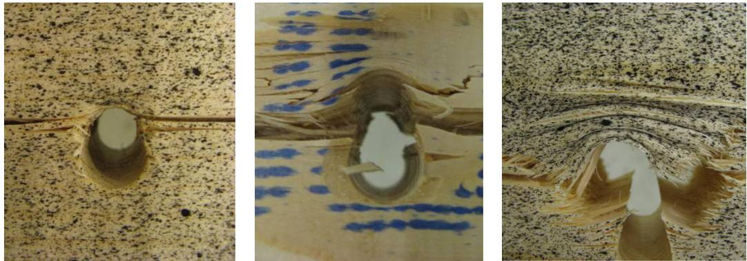
Figure 10: Fastener holes after failure of bending test specimens (series  $C_{i-j}$ )
