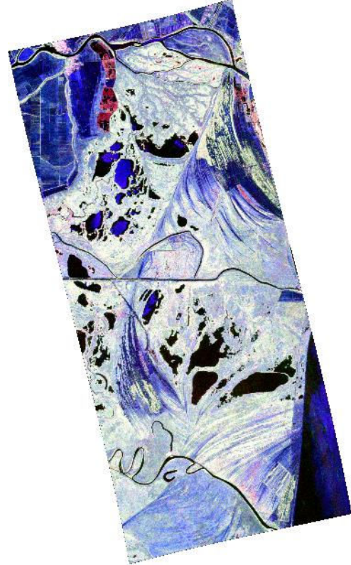
Figure 10: Optic image (top) and Pauli decomposition of the PolSAR data (bottom), rectified versions
