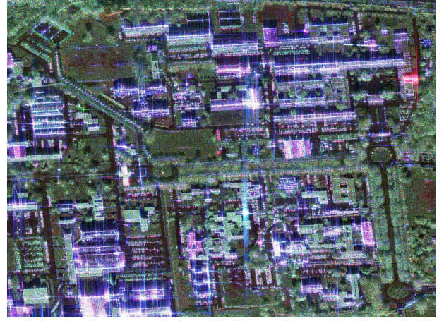
Figure 3. Toulouse, RAMSES POLSAR data, X-band, 1500 \times 2000 pixels: amplitude color composition of the target vector elements k_1 - k_3 - k_2 .
