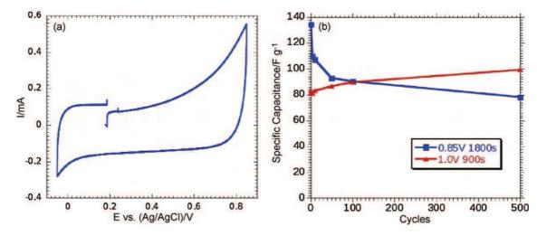
**Fig. 4.** CV of  $MnO_2$ -coated Ni nanorods (single-step method, 1 V for 900 s) in K<sub>2</sub>SO<sub>4</sub> 0.1 M (a). Evolution of capacitance upon cycling of an  $MnO_2$ -coated Ni nanorods electrode (b). Deposition performed by single-step potentiostatic method at 1.0 V for 900 s (triangles,  $m_{MnO_2} = 0.0177 \text{ mg}$ ) and at 0.85 V for 1800 s (squares,  $m_{MnO_2} = 0.0545 \text{ mg}$ ).
