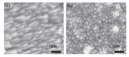
Fig. 5. MnO<sub>2</sub> deposited by two-step potentiostatic pulse method at 0.85 V for 3600 s (a) and 7200 s (b) on Ni nanorods.
