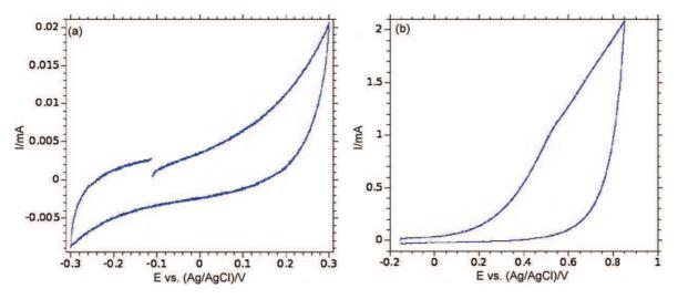
Fig. 2. CV measured of raw Ni nanorods in K<sub>2</sub>SO<sub>4</sub> 0.5 M to evaluate its capacitance (a) and its stability in a larger potential range (b).
