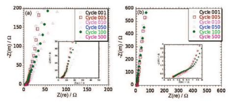
Fig. 7. EIS analyses upon cycling were performed on Ni nanorods coated by MnO<sub>2</sub> by single-step method (at 0.85 V for 900 s (a) and by two-step potentiostatic pulse method for 7200 s (b)).
