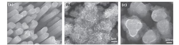
Fig. 1. SEM micrograph of raw Ni nanorods (a) used as substrate for the electrodeposition of MnO<sub>2</sub> and MnO<sub>2</sub> electrodeposited at 1.0 V/Ag–AgCl for 3600 s (b) and at 0.85 V/Ag–AgCl for 1800 s (c) on Ni nanorods.
