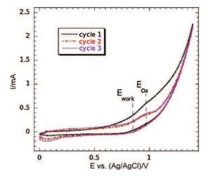
Fig. 3. CVs performed in the platting solution using a Ni nanorods substrate.
