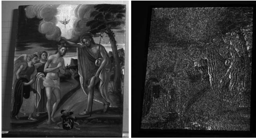
Figure 4: Left camera, after beam removal: initial image capture (left) and projected speckle pattern on the luminance-compensated image (right)
