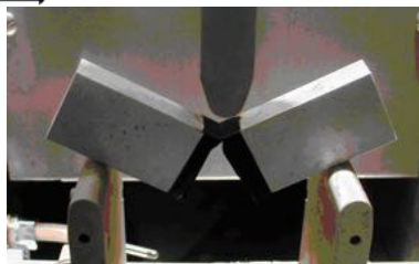
Three points bending test using a non homogeneous sample
