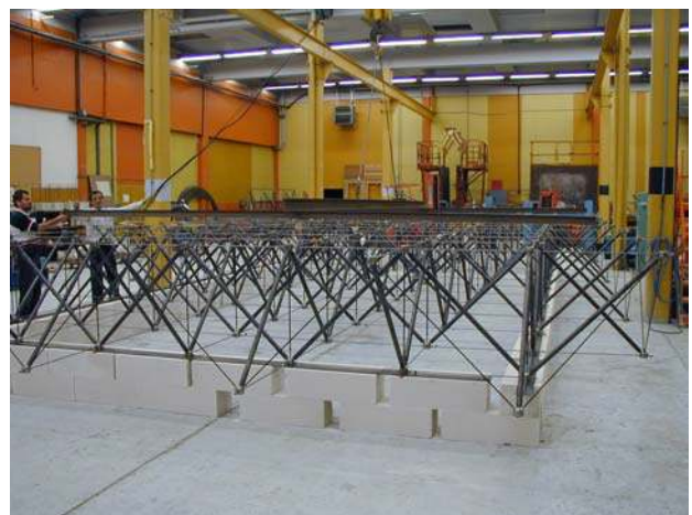
Figure 1: Double layer tensegrity grid. (Tensarch project)
