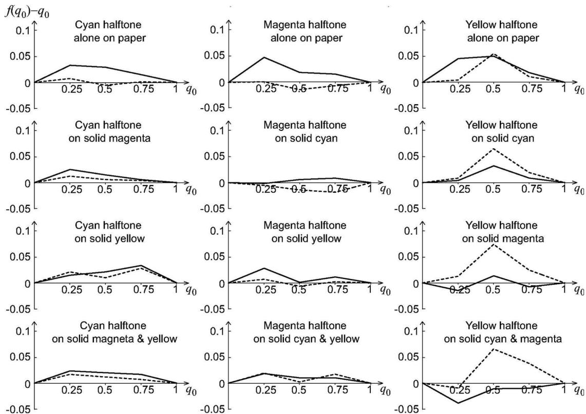
**Fig. 4.** Dot gain curves (difference between effective and nominal ink coverages as a function of the nominal ink coverage for a single halftoned ink) calibrated in reflectance mode (dashed lines) and transmittance mode (continuous lines). The 12 graphs correspond to cyan, magenta, or yellow halftones printed either alone on paper or superposed with a solid ink layer composed of the second ink, the third ink, or the second and third inks.
