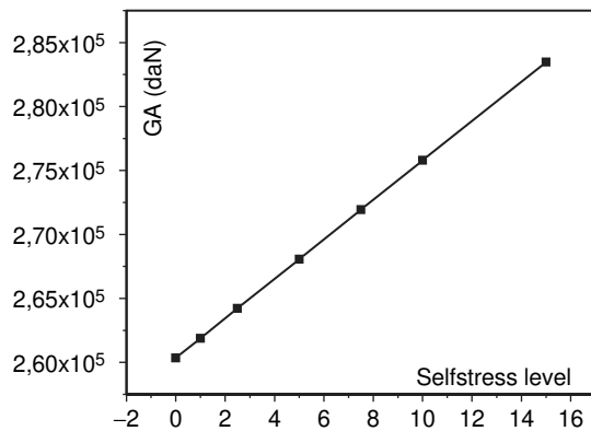
Figure 13. Equivalent shearing rigidity GA.
