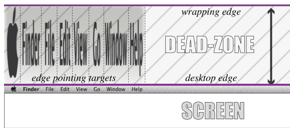
Figure 2. Wrapping dead zone (right) and expansion of targets located on the screen edge (left).
