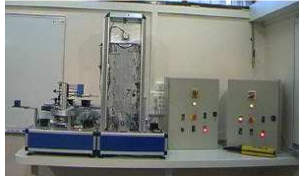
Fig 3: Our automation platform: a vertical store driven by two PLCs.
