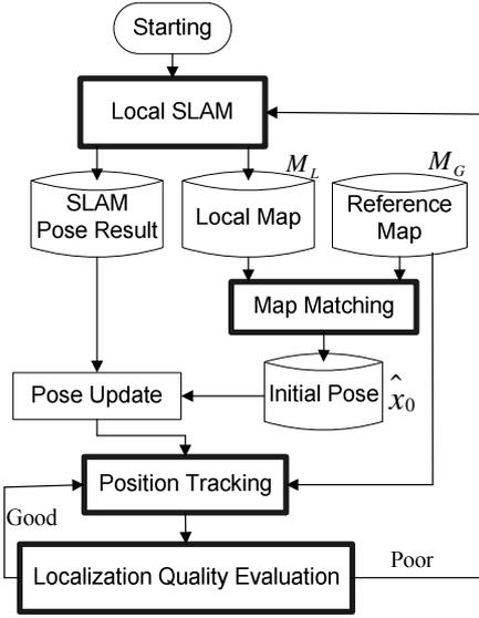
Figure 1. Architecture of the Localization System
