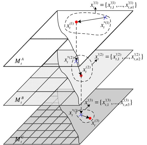
Figure 2. Pyramid grid-map based coarse-to-fine refining strategy
