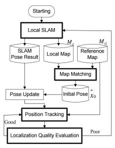
Figure 1. Architecture of the Localization System
