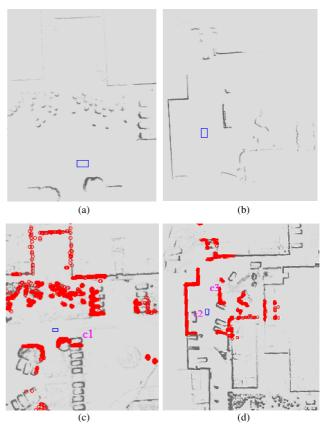
Figure 6. Experiment results of AGV: (a) Local map from A; (b) Local map from B; (c) localization result A; (d) localization result B.
