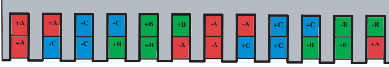
Figure 6. Double-layer windings distribution for a three phases machine with 12 slots and p = 1 .
