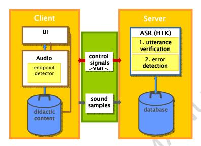
Figure 1. Schematic representation of the *Dutch-CAPT* system.
