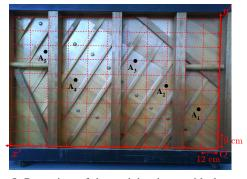
Figure 5: Rear view of the upright piano, with the mesh for modal analysis (in red) and the locations of the five accelerometers (in black).
