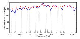
Figure 9: Typical bank-filtering analysis of a reconstructed impulse response between 550 et 1150 Hz (acoustical excitation). —: Fourier spectrum of the impulse response at point  $A_2$ . •: modes estimated by ESPRIT (modal amplitudes and frequencies). ···: amplitude responses of the narrow pass-band filters.
