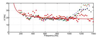
Figure 12: Average modal spacing of the piano soundboard: measured at points  $A_1(\cdot)$ ,  $A_2(\Delta)$ ,  $A_3(\nabla)$ ,  $A_5(\cdot)$ , numerically calculated with a finite-element model of a homogeneous isotropic clamped plate (**•**) and theoretical for the same plate (**—**).
