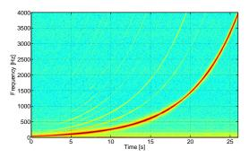
Figure 1: Spectrogram of the acoustical response of the *loud-speaker*, *room* system to an electrical signal. The distortion appears as successive harmonics of the swept-sine. The spectrogram is calculated with FFT over overlapping windows of 0.1 s with an 50% overlap.
