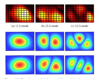
Figure 13: First three modal shapes of the upright piano soundboard: measured (first line), numerical (FEM) after replacement of the ribbed zone by a homogeneous isotropic equivalent plate (middle line), numerical (FEM) for the ribbed board without bridges (bottom line).
