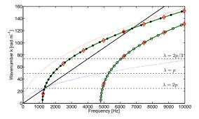
Figure 17: Relations of dispersion for flexural waves in the orthotropic plate ( $\cdots$  along x and  $\cdots$  along y), in the air (—) and for the two first waveguide modes (--- and --) of the waveguide between the second and third ribs. We add the discretes values corresponding to the waveguide modes (1, n) in  $\bullet$  and (2, n) in (o), together with the supposed perfectly harmonic partials of the  $\mathbf{D}_{\mathbf{6}}^{\sharp}$  strings in  $\diamond$ .
