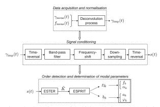
Figure 4: Block diagram of the high-resolution modal analysis method (after (Ege et al. 2009))
