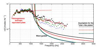
Figure 11: Modal densities of the board measured at points  $A_1(\cdot)$ ,  $A_2(\Delta)$ ,  $A_3(\nabla)$ ,  $A_5(*)$  and calculated for the first waveguide mode (1,n) of the corresponding inter-rib space (—, with the corresponding color). Asymptotic values of the modal densities of the inter-rib plates (–, with the corresponding color). Theoretical modal density of the homogeneous isotropic equivalent clamped plate (–·–), see next section.
