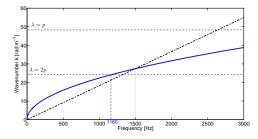
Figure 14: Dispersion curves in the isotropic plate (—), and in air (– –). The critical frequency of radiation of the plate is  $\approx 1500$  Hz. At  $\approx 1160$  Hz, the half-wavelength  $\lambda/2$  is equal to the average distance *p* between two consecutive ribs.
