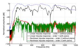
Figure 3: Nonlinearities of the two systems {*loudspeaker, room*} and {*loudspeaker, piano, room*}. The distorsion rate is comparable in both situations.
