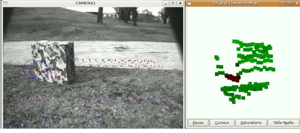
Fig. 6. Internal view of the experimentation. Our vehicle AROCO in a real outdoor environment. On the left : the camera picture with projected state points. On the right : the DEM.
