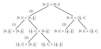
FIG 2. Binary tree labeled with the sequence of cutting directions (2, 1, 2, 2) corresponding with the dyadic partition represented in Figure 1.
