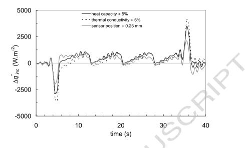
Fig. 5: Difference between the fixed and estimated heat flux
