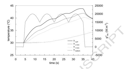
Fig. 3: Incident heat flux and computed temperature in the inoxidable mass (2D model).
