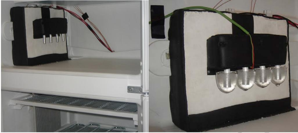
Fig. 5: Final assembly photographs of the ice maker prototype.
