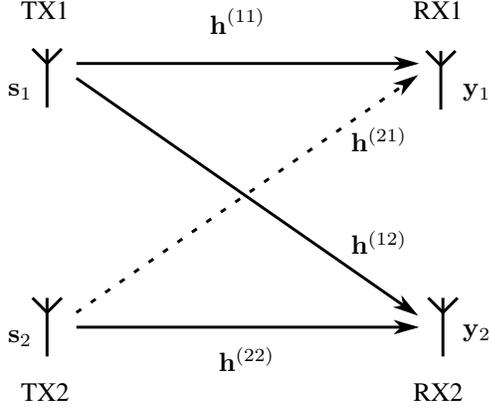
Fig. 1. Unbalanced cognitive interference channel model
