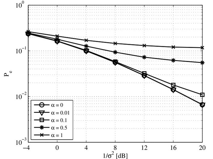
Fig. 7. Comparative probability of bit error ( $P_e$ ) for the MMSE equalizer for the secondary (VFDM) system with varying interference levels  $\alpha = \{0, 0.01, 0.1, 0.5, 1\}$  ( $N = 64$ ,  $L = 16$ ).
