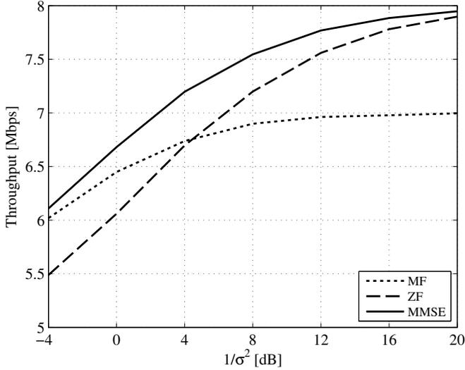
Fig. 5. Comparative throughput  $T$  for the MMSE, ZF and MF equalizers for the secondary (VFDM) system ( $N = 64$ ,  $L = 16$ ,  $\alpha = 0$ ).
