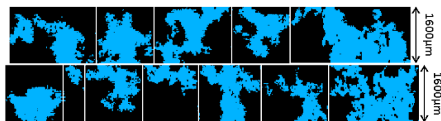
Fig. 15. Examples of CIP shadow images as observed at roughly 6 km altitude during the 16 August flight.
