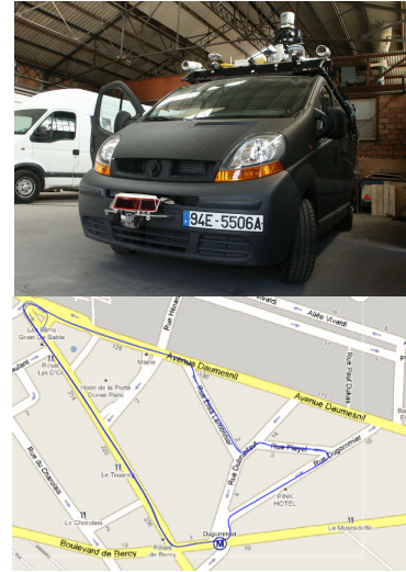
Fig. 10. On the top the test vehicle with the lidar sensor in front. On the bottom, the track follow by the vehicle
