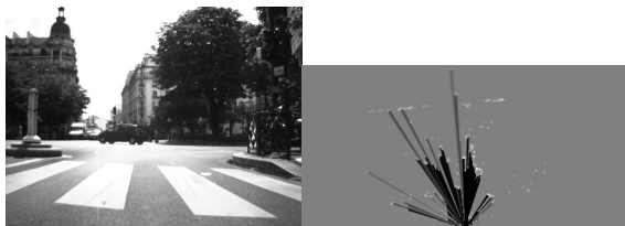
Fig. 4. Multi-echo sensor model: on the left the camera view of the scene and on the right the SG projected in a Cartesian frame, white cells are occupied, black are free, and gray are unknown.
