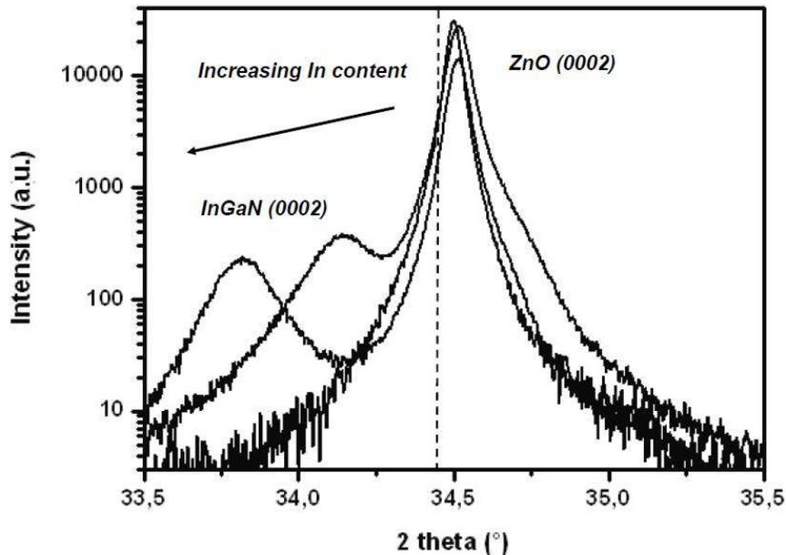
Figure 4. XRD  $2\theta$ - $\omega$  scans of the (0002) peak for ZnO/Si and the InGaN/GaN/ZnO/Si with varying In contents. The dashed line shows the peak position ( $34.43^\circ$ ) for a ZnO powder reference sample.
