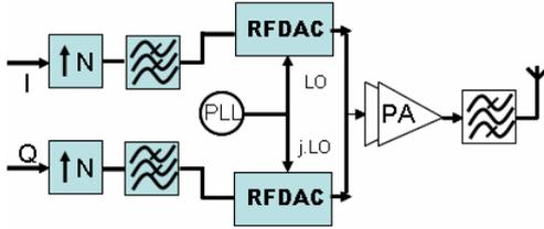
Fig. 2 Digital mixing architecture
