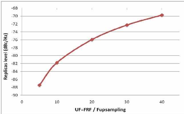
Fig. 7 Impact of up-sampling frequency on replicas level
