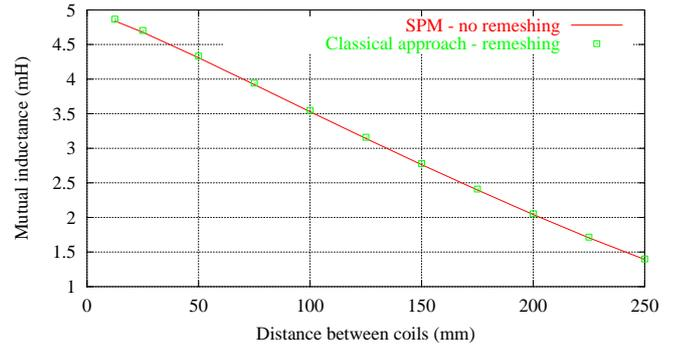
Fig. 2. TEAM problem 17: Mutual inductance as a function of distance between the main coil and a search coil.
