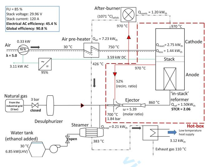
Figure 9. Detailed flow-sheet with ethanol feeding
