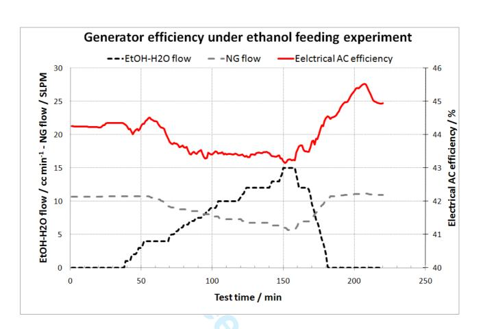
Figure 21. Generator electrical AC efficiency behaviour during the EtOH experiment
