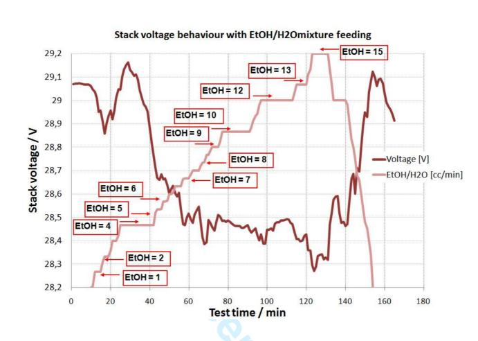
Figure 16. Behaviour of stack voltage during the EtOH/H2O feeding experiment
