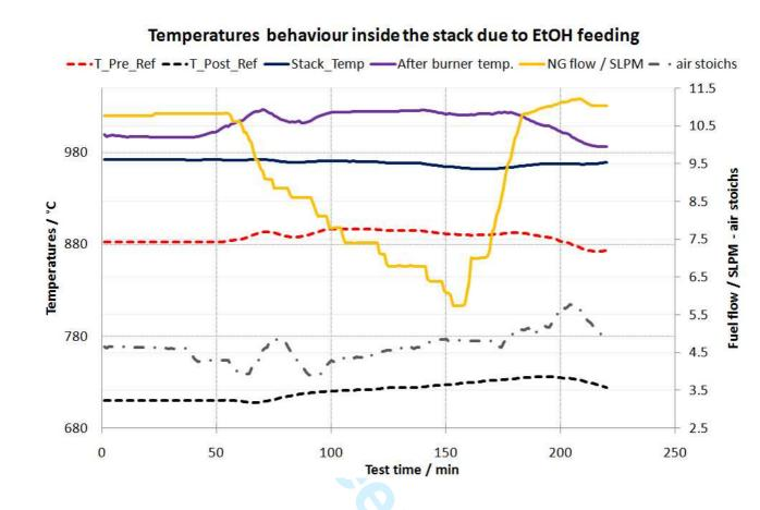
Figure 20. Generator temperatures behaviour during the ethanol experiment
