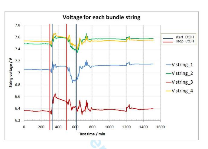
Figure 17. Comparison of string voltage during the EtOH/H2O feeding experiment
