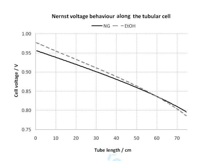
Figure 10. Comparison of the calculated Nernst voltage along the fuel channel (cell tube length) for both natural gas and ethanol feeding
