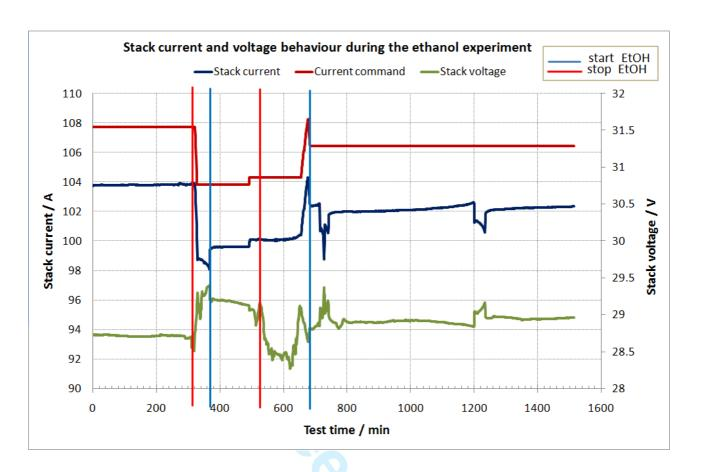
Figure 18. Stack voltage and current behaviour during the EtOH experiment
