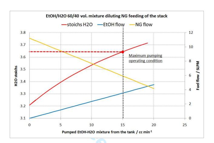
Figure 15. Water stoichiometry in the NG/EtOH mixture reaching the stack
