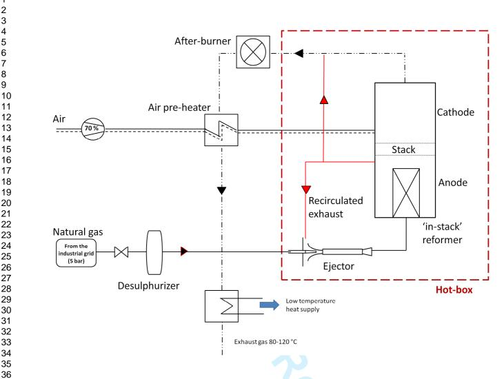
Figure 2. Basic BoP design of the SOFC generator analyzed
