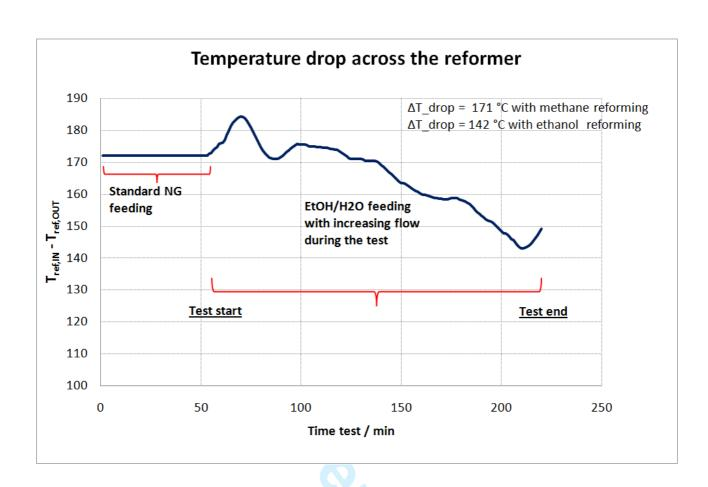
Figure 19. Reformer temperature drop during the ethanol experiment
