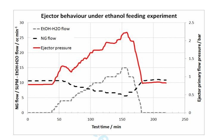
Figure 14. Ejector pressure increase during EtOH/H2O mixture feeding
