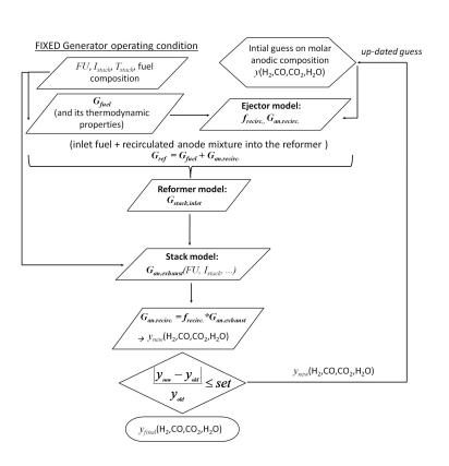
Figure 7. Schematic sheet describing the iteration step for determining the molar composition of the anodic exhaust 701x533mm (96 x 96 DPI)
