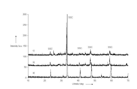
Fig. 8 XRD patterns of SSC cathode a) as prepared, b)after reduction 600°C-30min under H2 (2% in Ar), c) after C3H8/O2 exposure at 630°C during 3 hours 256x159mm (96 x 96 DPI)
