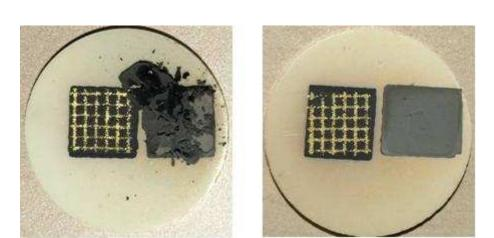
Fig. 14 Photographs of SCFC devices with a  $10\mu m$  (left) and  $40\mu m$  (right) thick anode, after tests shown in figure 13. 120x56mm (96 x 96 DPI)
