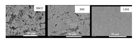
Fig. 6 SEM of BSCF, SSC and LSM cathodes (as prepared layers) 247x65mm (150 x 150 DPI)
