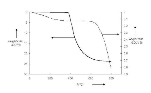
Fig. 2 Thermogravimetric analysis of NiO and GDC powders under hydrogen (2% in Ar), temperature rising rate 10°C/min. 224x131mm (96 x 96 DPI)
