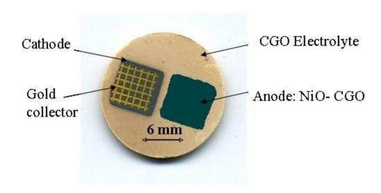
Fig. 1 SCFC prototype on GDC pellet with screen-printed electrodes. 131x65mm (96 x 96 DPI)
