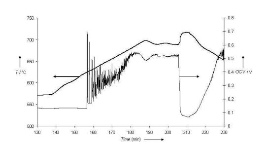
Fig. 9 Open Circuit Voltage time dependence of a Ni-CGO / CGO / LSM SCFC under Air-propane (C3H8/O2=0.55), versus time, with varying sample temperature 205x114mm (96 x 96 DPI)
