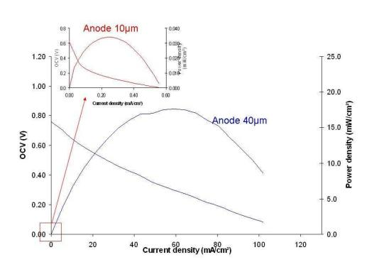
Fig. 13 Voltage-current characteristic of a Ni-CGO / CGO / LSM SCFC at 620°C (SCFC temperature) under Air-propane (C3H8/O2=0.53), with a total gas flow of 45l/h. Influence of anode thickness:  $40 \mu m$  in main curve,  $10 \mu m$  in insight.
