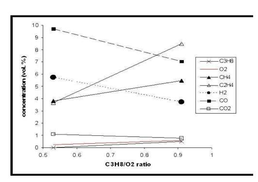
Fig. 11 Influence of C3H8/O2 ratio on outlet gas composition, during SCFC test, at 620°C with a total gas flow of 45l/h. 109x72mm (150 x 150 DPI)
