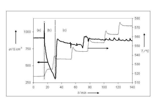
Fig. 4 Ni-GDC anode conductivity in air-propane mixture (C3H8/O2 = 0.66), versus temperature 205x123mm (96 x 96 DPI)
