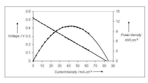
Fig. 10 Voltage-current characteristic of a Ni-CGO / CGO / LSM SCFC at 700°C (SCFC temperature) under Air-propane (C3H8/O2=0.55) 186x95mm (96 x 96 DPI)
