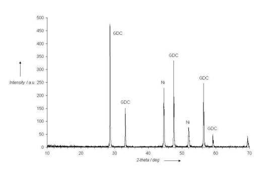
Fig. 3 XRD pattern of NiO-GDC anode after reduction 600°C-30min under hydrogen (2% in Ar) 256x159mm (96 x 96 DPI)
