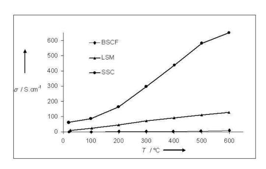
Fig. 5 LSM, SSC and BSCF cathodes conductivity in air, versus temperature 176x105mm (96 x 96 DPI)
