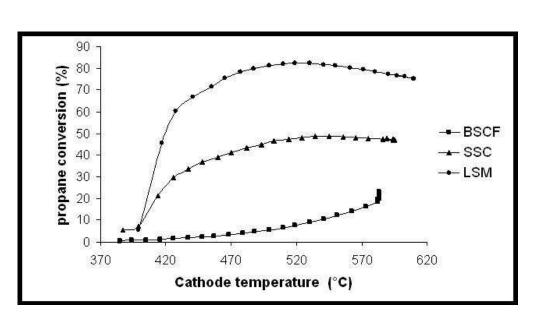
Fig. 7 Catalytic activity measured as propane conversion rate with a  $\mu$ GC-MS,of BSCF, SSC and LSM cathodes (powders in a fixed bed reactor)) 150x81mm (108 x 109 DPI)
