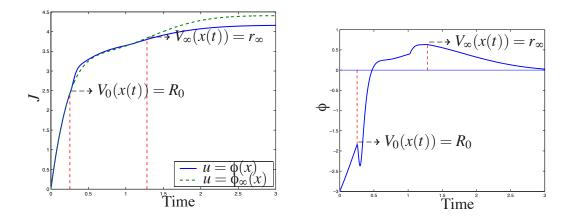
Fig. 1. Time-evolution of the cost function J with the controls Fig. 2. Time-evolution of the uniting controller  $\phi$ .  $\phi$  (in plain line) and  $\phi_{\infty}$  (in dashed line).
