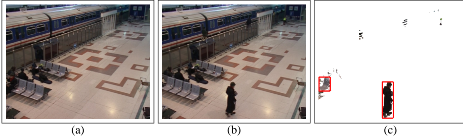
Fig. 1. Observations obtained with background subtraction and object isolation. (a) Reference frame. (b) Current frame (c) Result of background subtraction and derived object detection (two objects with red bounding boxes).
