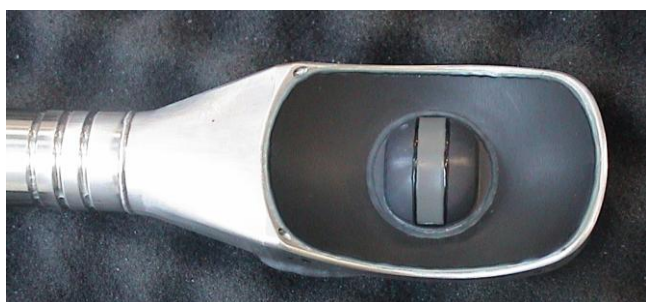
Figure 2 : EDAP Ablatherm HIFU technology
