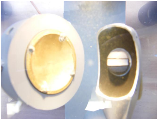
Figure 7 : Acoustic module of experimental setup. Transducers are placed at 90 degrees in a water tank; Zoom on confocal transducers during ultrasonic irradiation in degassed water
