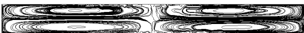
Figure 3: Streamlines of the steady-state acoustic streaming flow in the standing wave resonator of figure 1.
