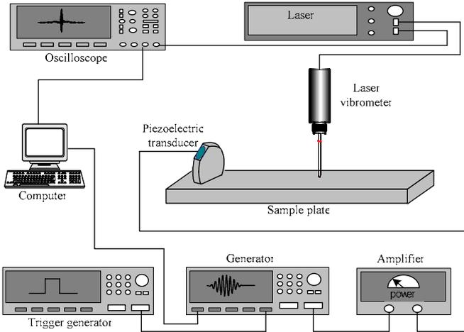
Figure 2: Experimental set-up used for the demonstration of the focusing properties of a “chaotic cavity transducer”.
