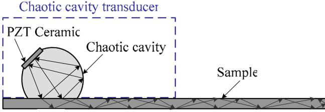
Figure 1: Principle of “chaotic cavity transducer”.
