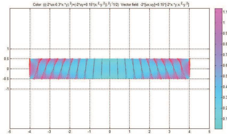
Figure 7: Shear stress field -  $B/H=8$  and  $\nu = 0.3$
