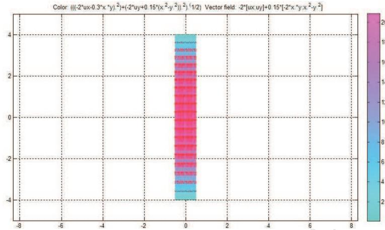
Figure 5: Shear stress field -  $B/H=1/8$  and  $\nu = 0.3$
