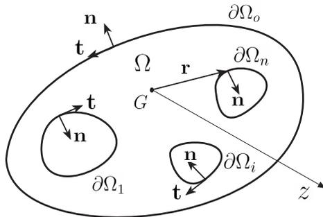
Figure 1: Multiply connected cross section of the beam
