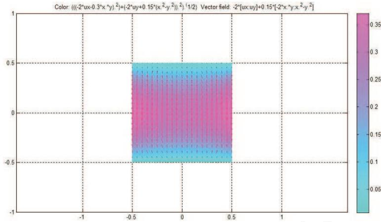
Figure 6: Shear stress field -  $B/H=1$  and  $\nu = 0.3$
