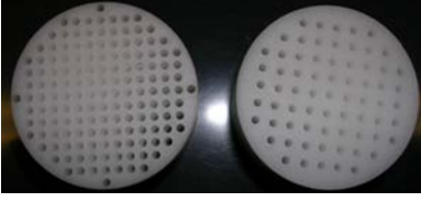
FIG. 10. (Color online) Photo of the simplified non-symmetric sample. Face A (left) includes all pores. Face B (right) only includes effective pores (without DE pores).
