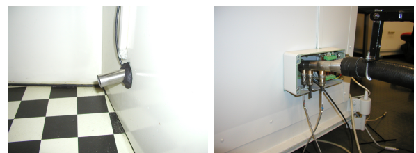
FIGURE 18 – Constant Volume Velocity source mounting : Monopole
