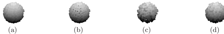
Fig. 3. Representation of aggregates with a spherical convex hull and different filling ratio: (a) full filling, (b) hollow filling, (c) random filling at 50%, (d) random filling at 75%
