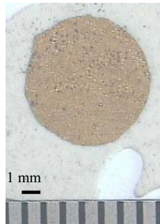
Fig.3 0-3 piezocomposite made with cubic PMN-28PT piezoelectric single crystal and TEGDM polymer (sample 1).
