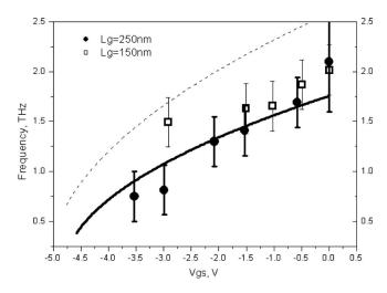
FIG. 4. Position of emission spectrum as a function of gate bias for AlGaN/GaN transistors with gate length 150 and 250 nm at drain to source voltage  $V_{ds}$ =4 V. Solid lines are calculations using Eqs. (1) and (2).
