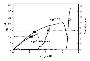
FIG. 2. Output characteristics and the emission intensity for sample 1 at gate biases  $V_{gs}$ =-3 V (squares) and for sample 2 at  $V_{gs}$ =-1 V (solid line).
