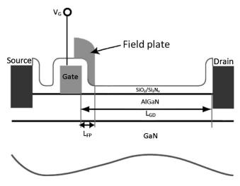
FIG. 1. Schematics of sample 2 with gate covered by a field plate.
