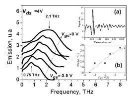
FIG. 3. The Emission spectra for GaN/AlGaN transistor ( $L_g$ =250 nm) at  $V_{ds}$ =4 V. Inset (a): the emission interferogram at  $V_{ds}$ =4 V and  $V_{gs}$ =-3 V. Inset (b): full width at half maximum of the spectra as a function of  $V_{gs}$  (dotted line is a guide to the eye).
