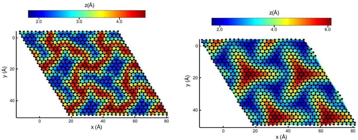
FIG. 3: Color map of the position of the C atoms in graphene along  $z$  (black dots). Initial gap set to 1.63 Å. FIG. 4: Same figure than Fig. 3 but for an initial gap of Blue (red) means near (far from) the SiC surface. Light 2.26 Å. crosses indicate the position of the Si atoms of the surface.
