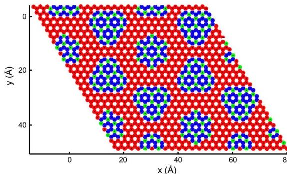
FIG. 7: Weakly stuck three-level structure of the graphene layer. Mean gap equal to 2.62 Å. Same color code than in Fig. 5.
