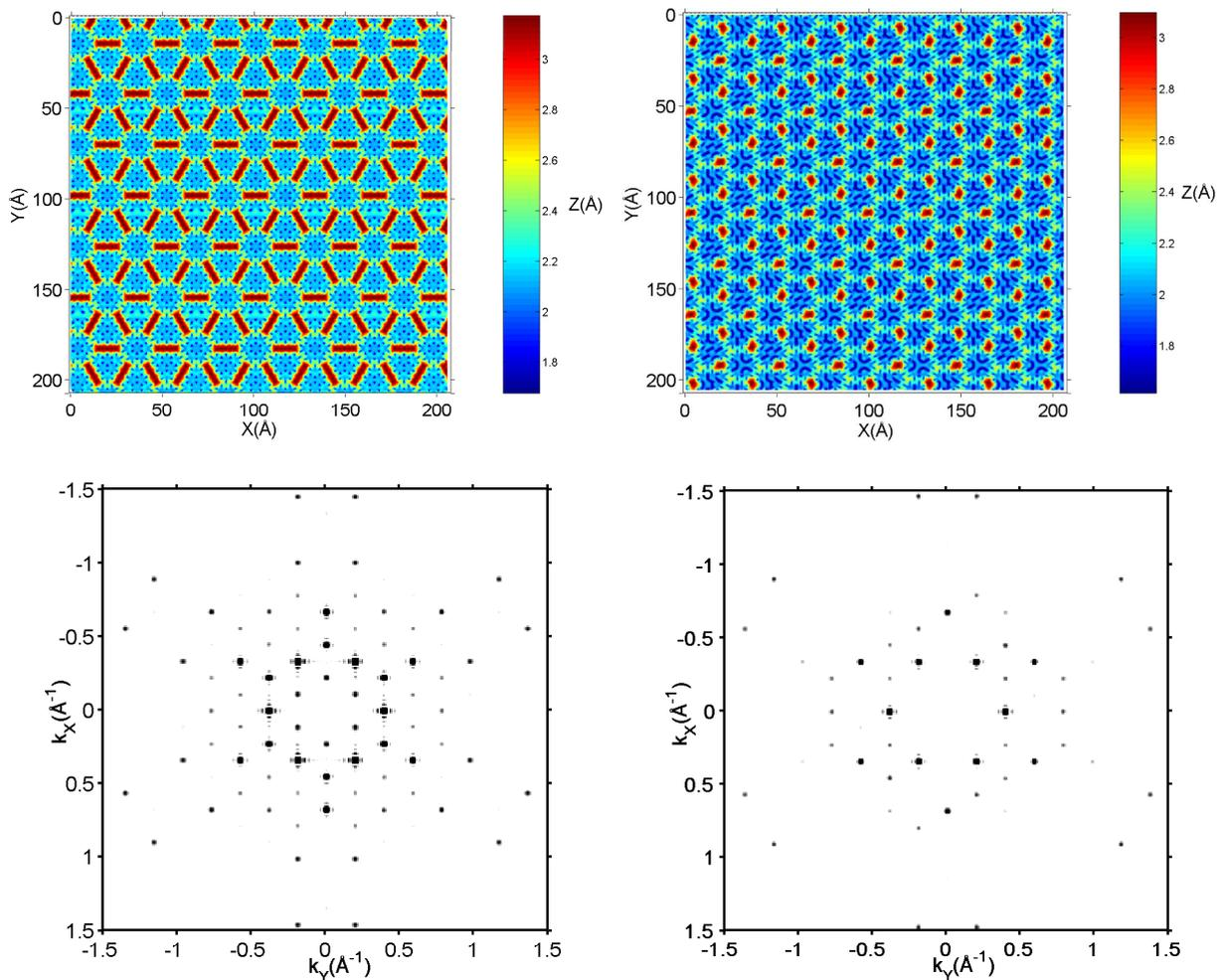
FIG. 12: Top: color map on the positions of C in graphene. Bottom: Fourier transform of the top color map, zoom at low  $k$  to emphasize the large scale order. Left: EDIP. Right: *ab initio*<sup>4</sup>.
