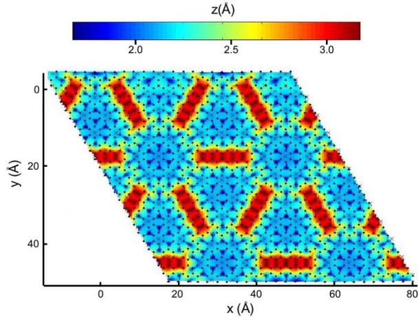
FIG. 10: Color map of the positions along  $z$  of the C atoms (black dots) in graphene. Most stable configuration. Blue (red) means near (far from) the SiC surface. Light crosses indicate the position of the Si atoms of the surface.
