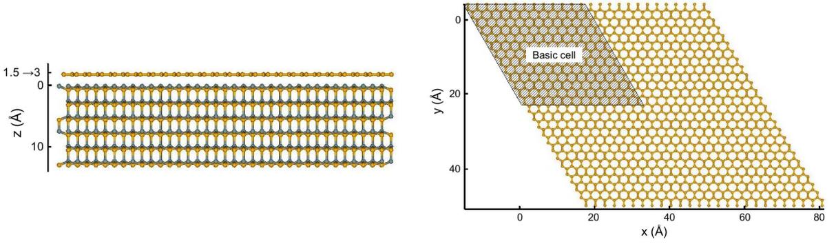
FIG. 1: Lateral (left) and top (right) views of the atomic system under study. The C atoms are colored in orange, the Si in grey. The delimitations of the basic cell are shown on the right view.
