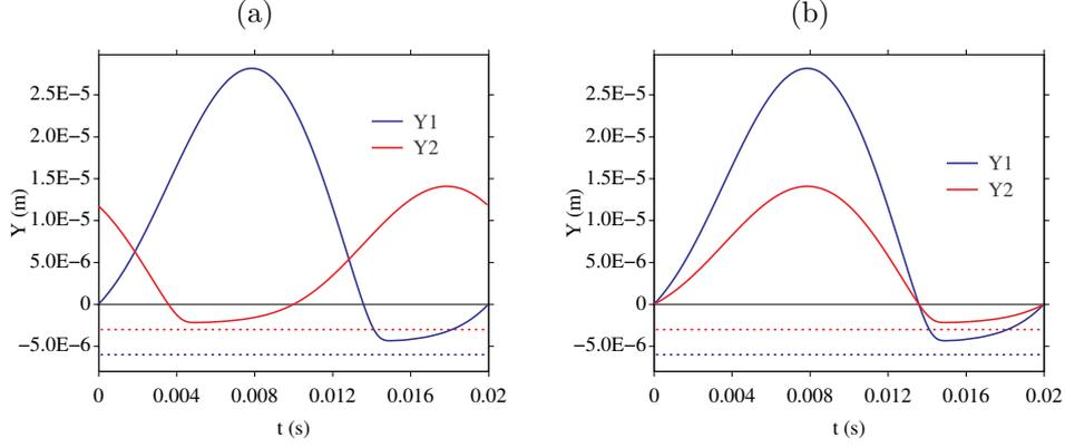
Fig. 9. Time history of  $Y_1$  and  $Y_2$  during one period, with  $\theta = 0.5$  (a) and  $\theta = 1$  (b): see theorems 5.1 and 5.2. Parameters: model 1 (3.5), sinusoidal forcing (3.7) with  $v_0 = 5 \cdot 10^{-3}$  m/s. The horizontal blue and red dotted lines denote the lower bounds  $-d_1$  and  $-d_2$ , respectively.
