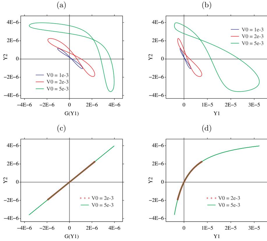
Fig. 11. Configuration space  $\Gamma_G$  (a-c) and  $\Gamma_I$  (b-d) with  $\theta = 0.5$  (a-b) and  $\theta = 1$  (c-d): see proposition 5.2. Amplitude  $v_0$  of the sinusoidal forcing (3.7):  $10^{-3}$  m/s,  $2 \cdot 10^{-3}$  m/s,  $5 \cdot 10^{-3}$  m/s.
