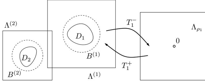
Figure 2: 2D-Sketch of a scatterer consisting of two parts  $D_1$  and  $D_2$ . The cylinders  $B^{(1)} = o_1 + B_{\rho_1/2}$  and  $B^{(2)} = o_2 + B_{\rho_2/2}$  are contained in the boxes  $\Lambda^{(1)}$  and  $\Lambda^{(2)}$ , respectively. The computational domain  $\Lambda_{\rho_1}$  is the reference domain for  $\Lambda^{(1)}$  and  $T_1^\pm$  transport functions between the two domains.
