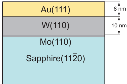
Figure 1: Schematic structure of the multilayer sample employed. The thickness of the Mo layer is 0.7 nm.
