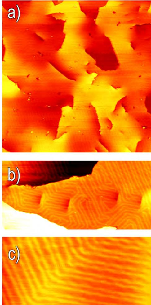
Figure 3: STM images of the Au(111) thin film surface (a) Large scale showing the presence of different defects ( $360 \times 360 \text{ nm}^2$ ). (b) Effect of a sequence of stacking fault ribbons on Au(111) reconstruction ( $130 \times 60 \text{ nm}^2$ ). (c) The reconstruction deviates from its unidimensional character and turns of  $120^\circ$  as in the herringbone reconstruction ( $60 \times 30 \text{ nm}^2$ ).
