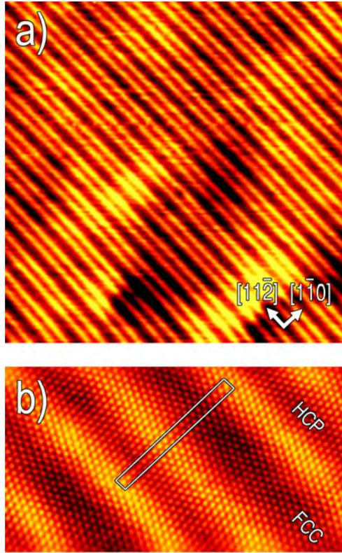
Figure 2: (a) Room temperature STM image showing the unidirectional reconstruction of the stressed Au(111) surface ( $85 \times 85 \text{ nm}^2$ ). (b) Drift compensated atomic resolution STM image, with the unit cell highlighted ( $15 \times 8 \text{ nm}^2$ ).
