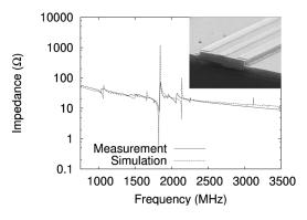
FIG. 2. Electrical response of a guided wave resonator (continuous line), compared to simulations (dashed line). Inset is a SEM view of a resonator with three fingers as its top electrode.
