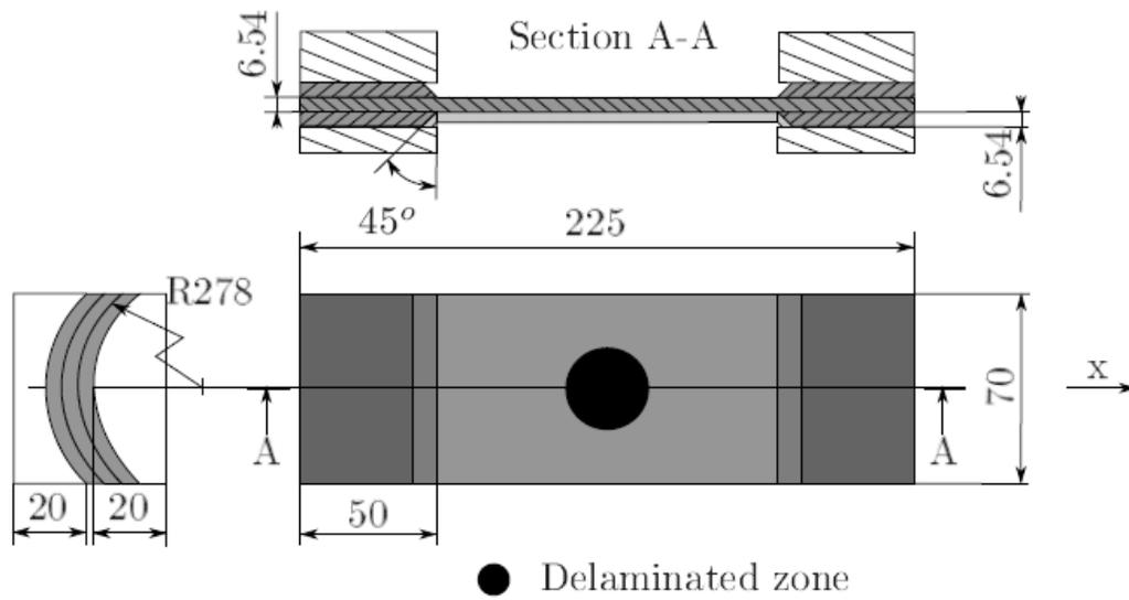
Figure 13 : Geometry of the tensile specimens
