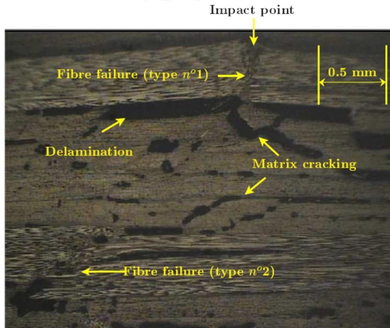
Figure 11 : Microscopic observation presenting the damage mechanisms observed
