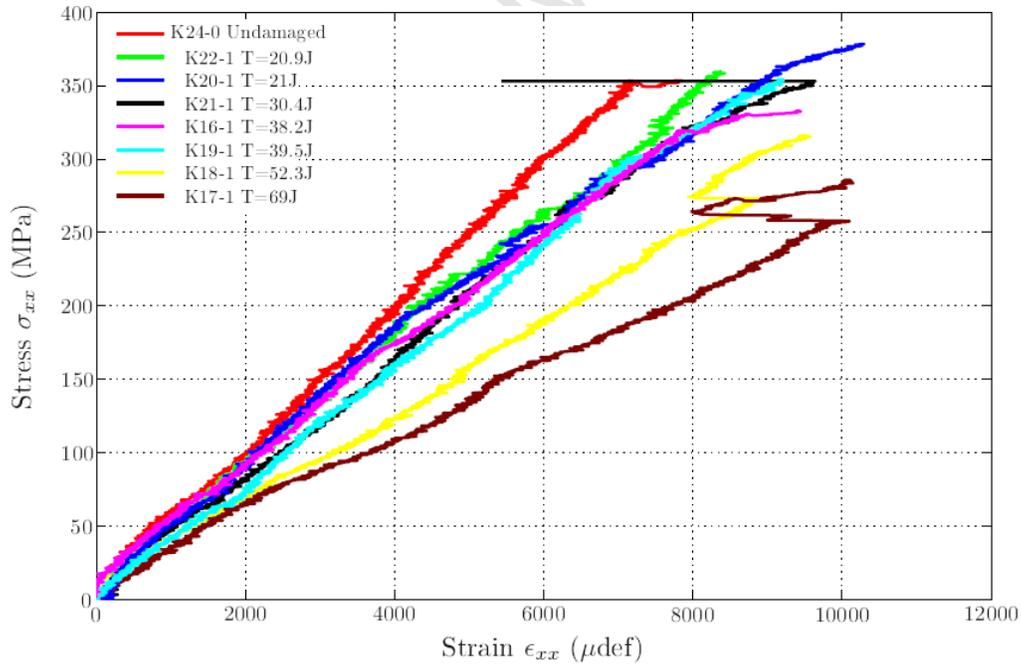
Figure 15 : Stress-strain curves corresponding to quasi-static tests on pre-impacted specimens
