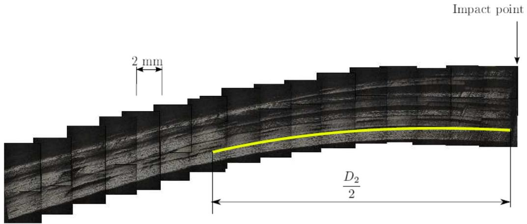
Figure 12 : Microscopic observation presenting the delamination observed
