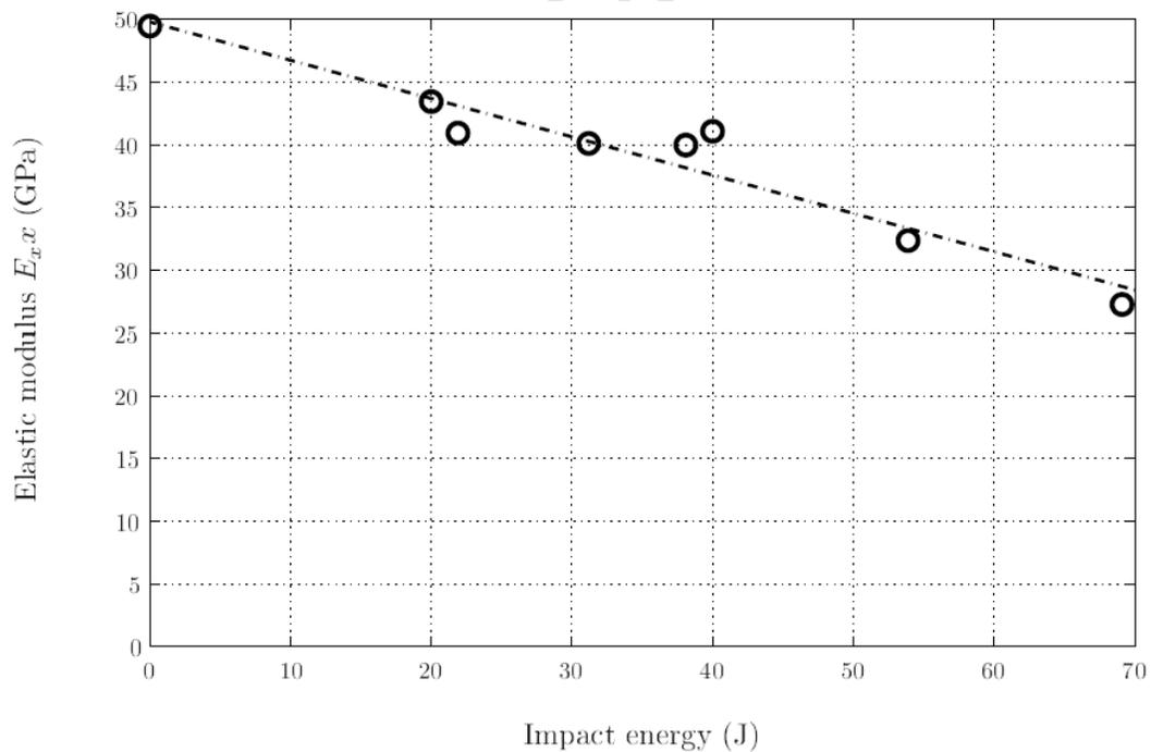
Figure 17 : Homogenized elastic modulus vs impact energy for quasi-static tests on pre-impacted specimens
