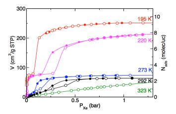
*Figure 1.* Experimental xenon adsorption isotherms in MIL-53 (Al). Open symbols: adsorption branch; filled symbols: desorption branch. Left scale: measured adsorbed volumes. Right scale: corresponding number of adsorbed molecules per unit cell. The low-pressure desorption branch at 195 K (hysteresis loop) has not been recorded, for technical reasons.
