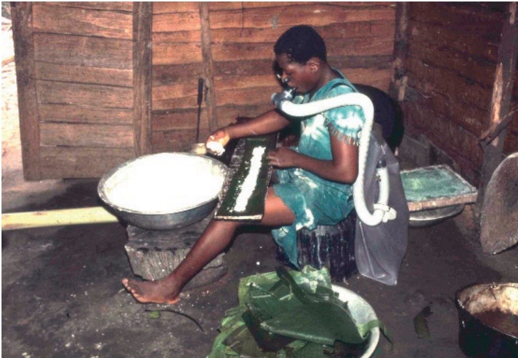
Figure 4 — A Douglas bag receiving the exhaled gas during a specific activity (here preparation of manioc) to determine the energy expenditure for calculation of the energy budget, in a village of southern Cameroon.
