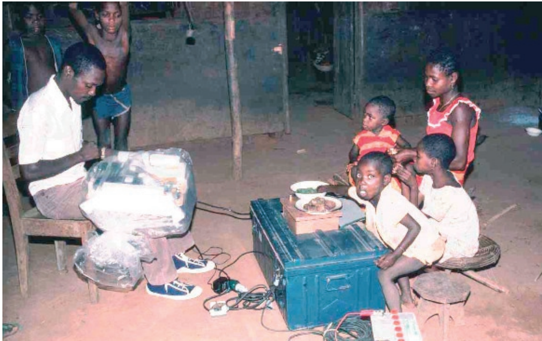
Figure 3 — An accurate measurement of the individual food intake in a communal dish. The dish is placed on a precision scale (one gram for 30,000 g) protected in a trunk with a thin PVC sheet and dryer. The operator, whose micro-computer is also protected from humidity, records the weight of each helping for each participant.
